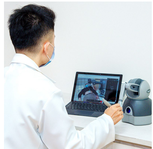
A physician uses a force feedback joystick to carry out remote robotic ultrasound scans.
