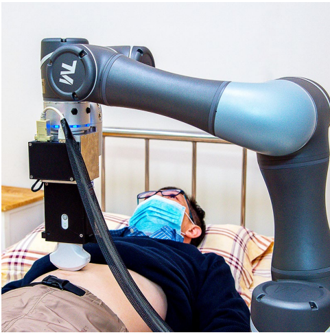
The robotic arm performs an abdominal ultrasound examination.
